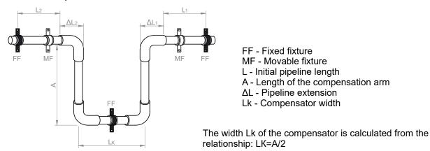
In case of placing the fixed support point PC on the segment, which is the width of the compensator Lk, to calculate the compensation arm A, it is necessary to take the equivalent length Le as the greater of the values L1 and L2: Le = max(L1, L2) and for this length find the equivalent elongation  $\Delta$ L, and then the length of the compensation arm A according to Table 1
