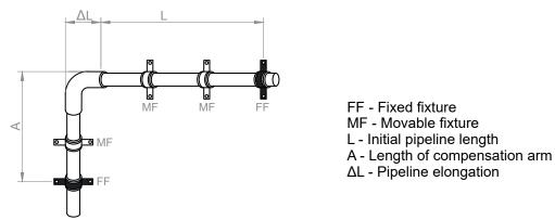
To calculate the compensation arm A, it is necessary to take the equivalent length Le=L and for this length determine the elongation value  $\Delta L$ , and then find the length of the compensation arm A according to table 1
